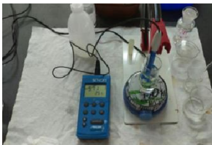
Slika 10. Prenosivi pH-metar, Handylab pH/LF, Schott Instruments GmbH.
