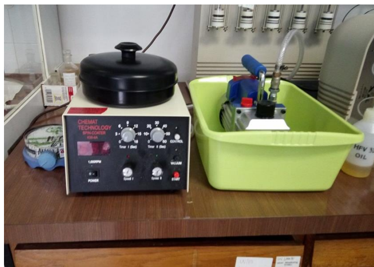
Slika 12. Spin coater , Chemat Technology.
