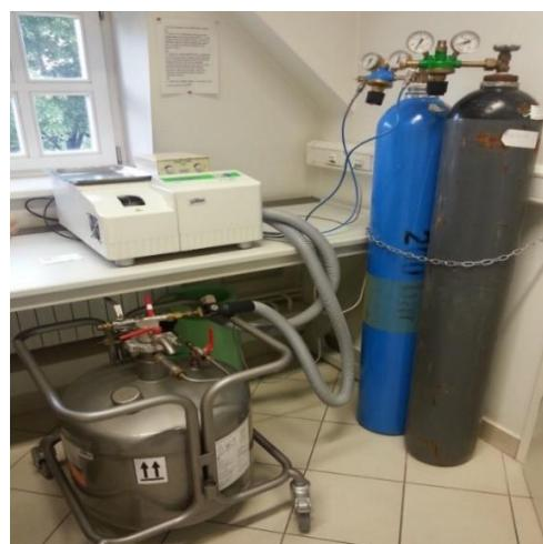
**Slika 15.** DSC instrument Mettler Toledo DSC 822<sup>e</sup>.
