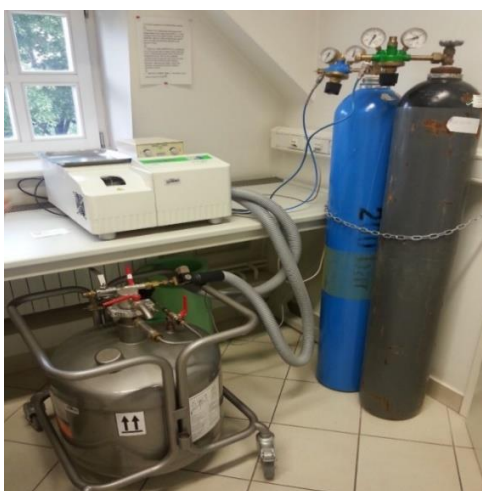
Slika 15. DSC instrument Mettler Toledo DSC 822 e .
