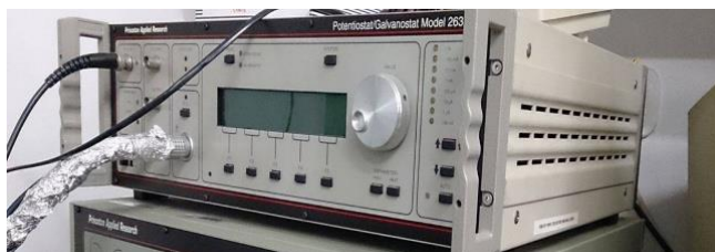
Slika 1. Potenciostat EG&G Princeton Applied Research, model 263A
