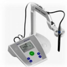
Slika 3.2. Mettler Toledo S20 SevenEasy pH metar [50]
