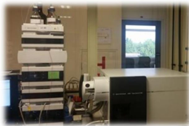
Slika 3.5. UHPLC Agilent Series 1290
