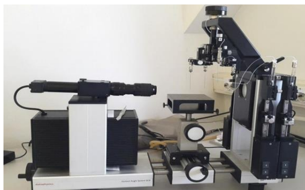
Slika 21. Goniometar DataPhysics OCA 20 Instruments, GmbH
