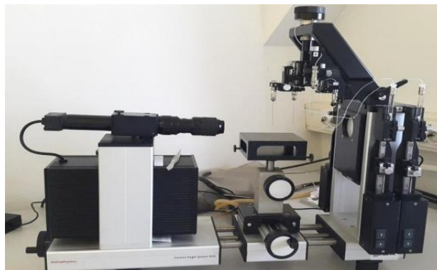
Slika 21. Goniometar DataPhysics OCA 20 Instruments, GmbH
