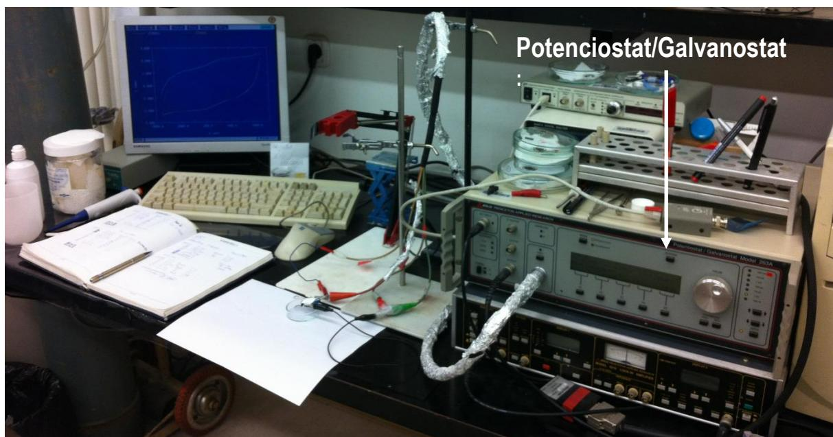
Slika 3.7. Potenciostat/Galvanostat: EG&G Princeton Applied Research, model 263A
