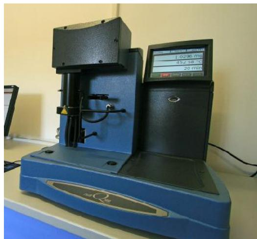
**Slika 14.** Termogravimetar, Q500 TA Instruments.
