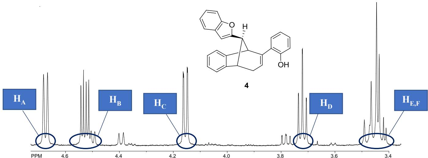
**Slika 7.** Alifatski dio <sup>1</sup>H NMR spektra fotoprodukta **4** (600 MHz) u CDCl<sub>3</sub>
