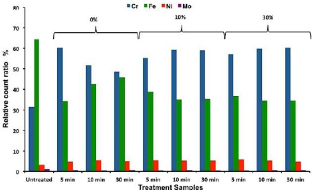
Figure 63: ToF SIMS isotope count (Fe, Cr, Ni and Mo) of untreated 316 SS (1) and treated samples of 316 SS in 0.5 M  $\text{H}_2\text{SO}_4$  with 0%, 10% and 30% glycerol additive at  $12.5 \text{ mA cm}^{-2}$  at 25
