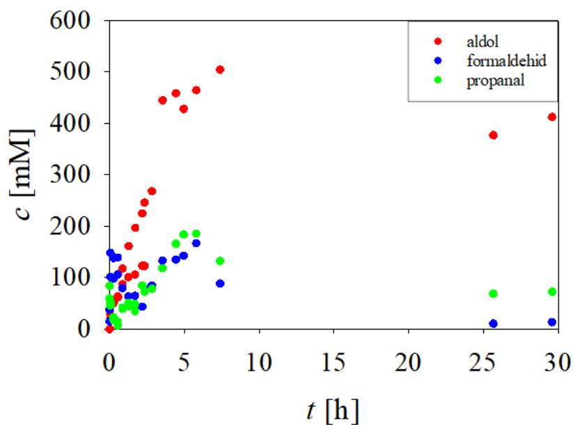
**Slika 4.11.** Utjecaj enzima FSA VarII na reakciju aldolne adicije u kotlastom reaktoru s dotokom ( $25\text{ }^{\circ}\text{C}$ ,  $50\text{ mM}$  pufer,  $\gamma_{\text{FSA}} = 60\text{ mg mL}^{-1}$ ,  $c_{\text{propanal}} = 55,43\text{ mM}$ ,  $c_{\text{formaldehid}} = 57,93\text{ mM}$ ,  $q_v, \text{propanal} (13,53\text{ M}) = 1,05\text{ }\mu\text{L min}^{-1}$ ,  $q_v, \text{formaldehid} (12,95\text{ M}) = 1,05\text{ }\mu\text{L min}^{-1}$ )
