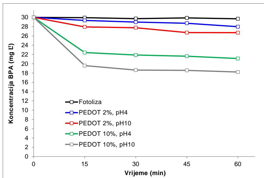
**Slika 4.5.** Testiranje adsorpcije BPA na fotokatalizatore TiO<sub>2</sub>-PEDOT (APS) u mraku (pH 4 i 10,  $\gamma(\text{BPA}) = 30 \text{ mg L}^{-1}$ ,  $\gamma(\text{TiO}_2) = 2,0 \text{ g L}^{-1}$ ) i razgradnja BPA izravnom solarnom fotolizom ( $\gamma(\text{BPA}) = 30 \text{ mg L}^{-1}$ )
