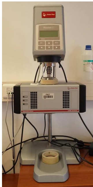
Slika 3.2.6.1. Reometar Anton-Paar, Rheolab QC [32]
