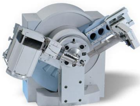
Slika 3-3-5 XRPD uređaj, PANalytical X'Pert Pro powder diffractometer , model PW3050/60
