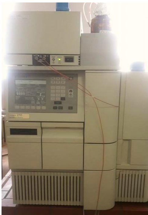
Slika 13. HPLC-DAD (Waters 2795 Alliance HPLC System with 2996 PDA Detector)
