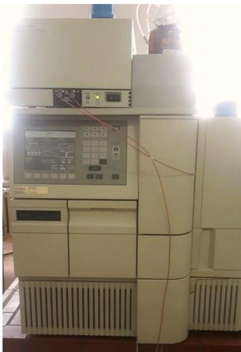
Slika 13. HPLC-DAD (Waters 2795 Alliance HPLC System with 2996 PDA Detector)
