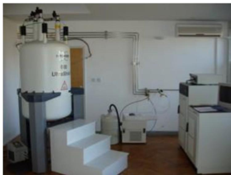
Slika 3.8:<sup>1</sup>H NMR Spektrometar Bruker Avance 300
