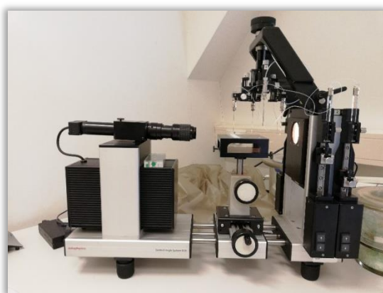
Slika 21. Goniometar DataPhysics OCA 20 Instruments, GmbH
