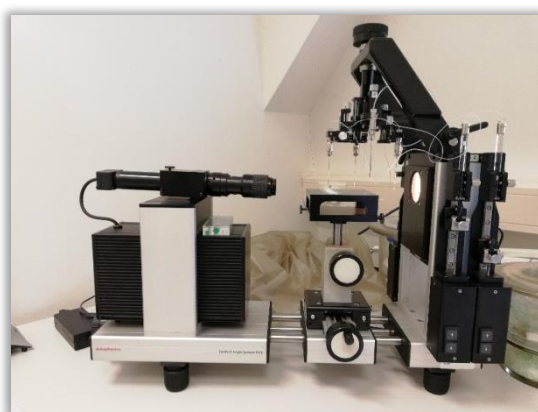
Slika 21. Goniometar DataPhysics OCA 20 Instruments, GmbH
