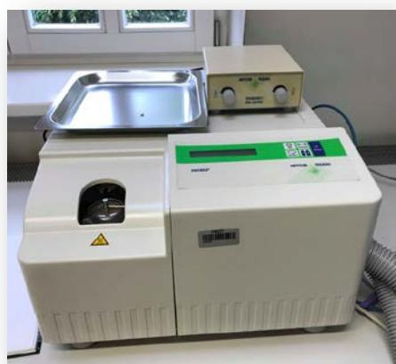
**Slika 17.** DSC analizator 822<sup>e</sup>, Mettler Toledo
