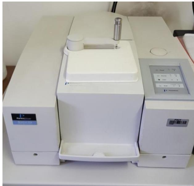
Slika 3.5 Spektrofotometar Perkin Elmer Instruments, Spectrum One.
